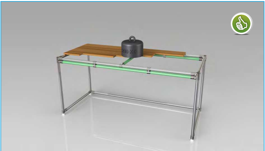
1. Double horizontal pipe with additional horizontal support
